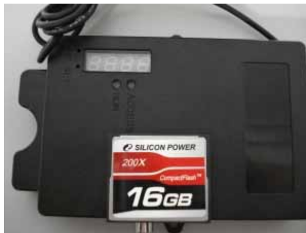
Figure 2. Camera control unit embedded inside e-JIKEI Light (Images are coded with secret key and recorded)
